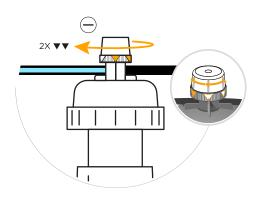
**Ready!** Since the soil is moist, the Tropf-Blumat may not discharge any water. Watering does not begin until the soil is dry. Now make the setting for every single Tropf-Blumat.
