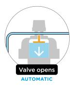
Every Tropf-Blumat is a sensor which controls watering of the plant. The sensor reacts directly to the moisture of the soil. If the soil becomes dry, a valve opens and watering begins. When the soil is sufficiently moist again, the release of water is automatically stopped.
