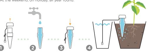
Blumat Classic is the reliable watering system for indoor plants. The water is tributed into the soil via the clay cone.
